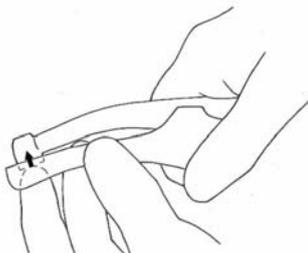
1. While one hand holds the assembly, the other hand holds the middle part of the handle of the device with the thumb and middle finger, while pushing the turbine head through the ring with the index finger to dislodge it from its location.
