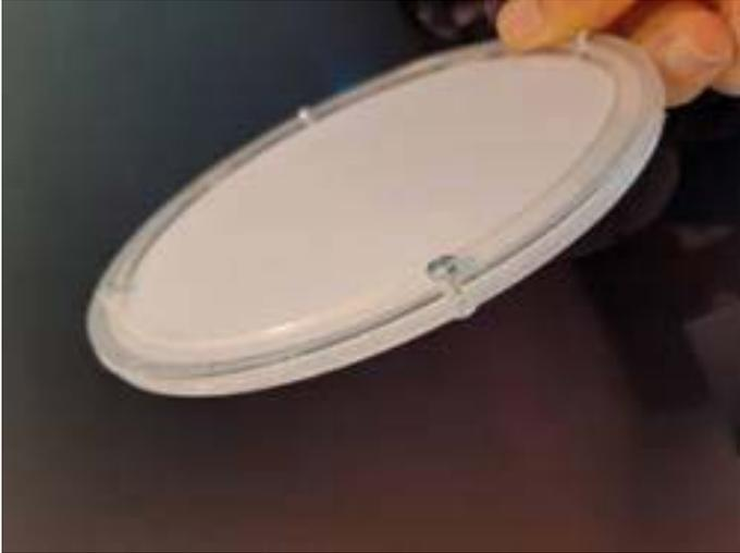
With the intention of capturing the aerosol particles produced by the turbine, a Whatman disc of cotton cellulose qualitative filter of 15 cm. in diameter and 0.18 mm. thick, mounted on a circular methacrylate frame is available. This frame fits into an infundibulum connected to a suction system that sucks the air through the filter at a rate of 216 l / min. All air flow measurements have been performed with an air column float flowmeter "ASA P13-2800".
